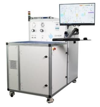
Potentiostats with EIS allow analysis of the cells of fuel cells, electrolyzers and consequently help the end customer to optimize and improve the efficiency of their systems.
