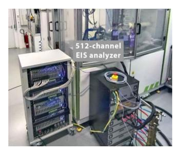
MegaEIS is a Multi-Channel EIS Analyzer for Hydrogen Fuel Cell and Electrolyzer Stacks. Designed for Hydrogen with High Currents and Peak Performance. Equipment deployed at the University of Chemnitz can handle voltage up to 600 V and currents up to 650 A (16 kW) and measure 512 channels simultaneously up to 100 kHz. The latest versions of MegaEIS can handle voltage up to 1000 V and currents up to 2000 A and measure 1024 channels simultaneously up to 100 kHz.
